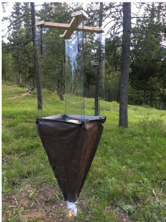
**Figure 2.** Flight intercept trap design. Traps consisted of two 24”x18” acrylic sheets cut half way up their longitudinal axis and slid together, a wooden top support, and a tarp funnel below with a collection container. Collection containers were filled with cut pieces of No-pest® Strip2.
