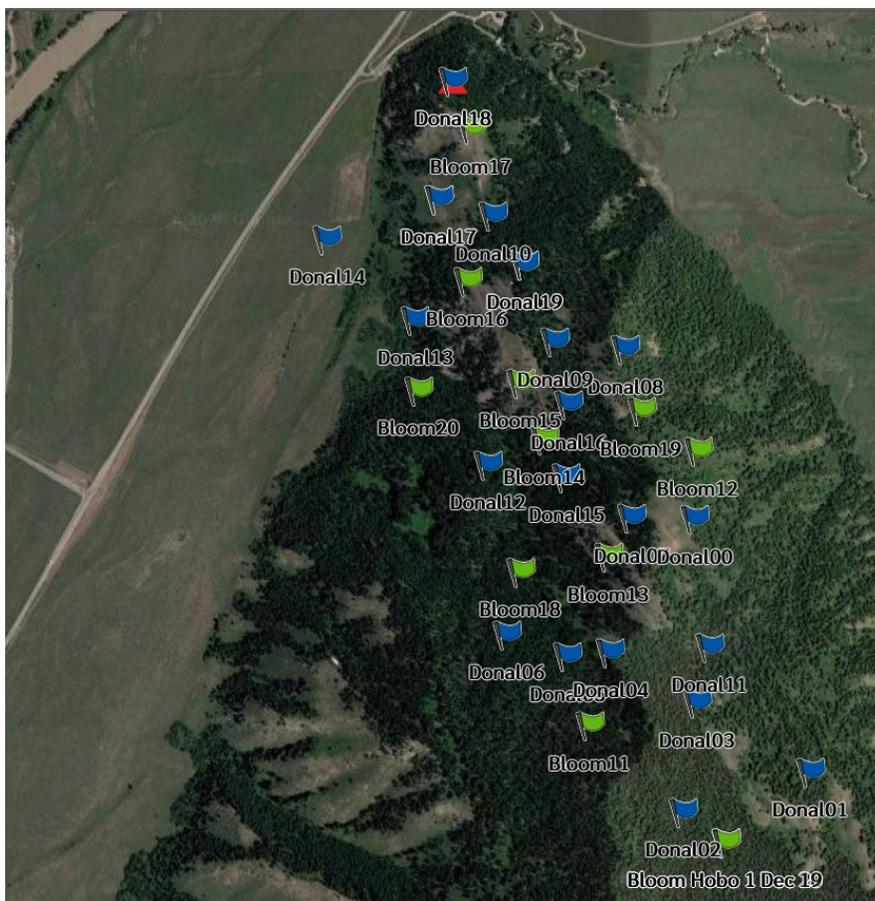
**Figure 2.** Close up view of northern Blacktail Butte where we have installed 36 climate sensors. Each station contains at least one sensor measuring ambient air temperature. Certain climate stations located at each of the six core phenology sites include a temperature sensor in the soil, pollinator collections, and game cameras for wildlife sightings and snow depth validation.
