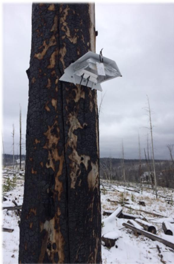
**Figure 2.** HOBO temperature data logger and housing unit at the Wind River planting unit.
