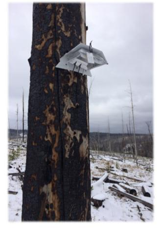
**Figure 2.** HOBO temperature data logger and housing unit at the Wind River planting unit.
