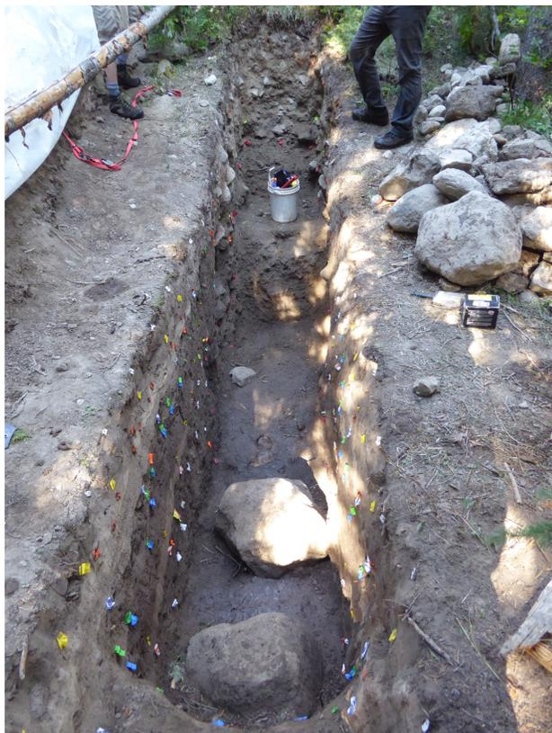
**Figure 4.** Trench B, which exposed the Teton fault on the lower slope of a 3.5 m high scarp. View is to the east-northeast. South wall (left) exposes well stratified, charcoal-rich sequence of alluvial sediments and paleosols.
