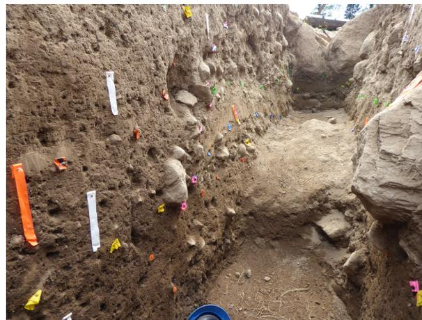
**Figure 3.** Trench A, which exposed the Teton fault across a low scarp (<1.5 m). View is to the west-southwest.
