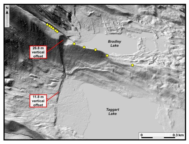
**Figure 3.** Samples collected for cosmogenic <sup>10</sup>Be surface exposure ages of moraine boulders (yellow dots) and vertical fault offsets on lateral moraine and valley bottom near Taggart Lake. LiDAR data provided courtesy of Kathy Mellander at Grand Teton National Park.
