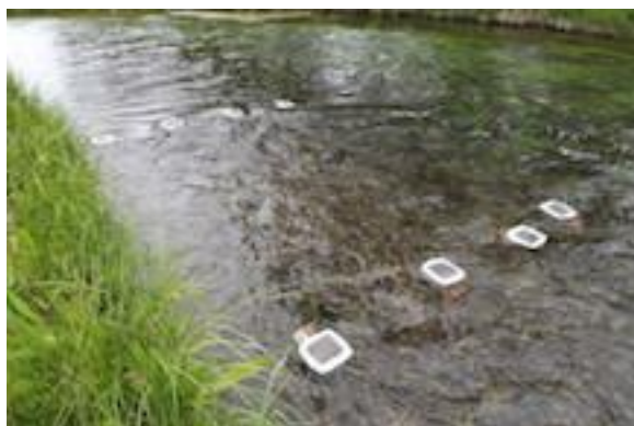
Figure 4. Eight Hydropsyche collection tiles within anchored experimental chambers.
