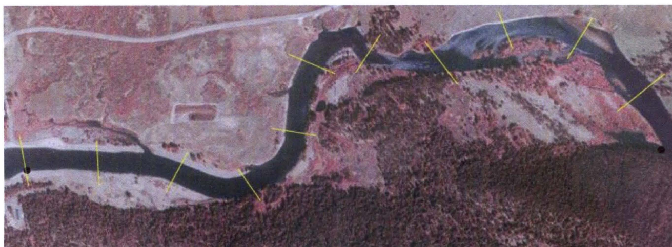
Figure 1. An example of site selection design, consisting of a series of 11 transects placed at 250 m separation. The site (11 transects) covers a distance of approximately 40 times the river width, based on EPA EMAP sampling protocol.
