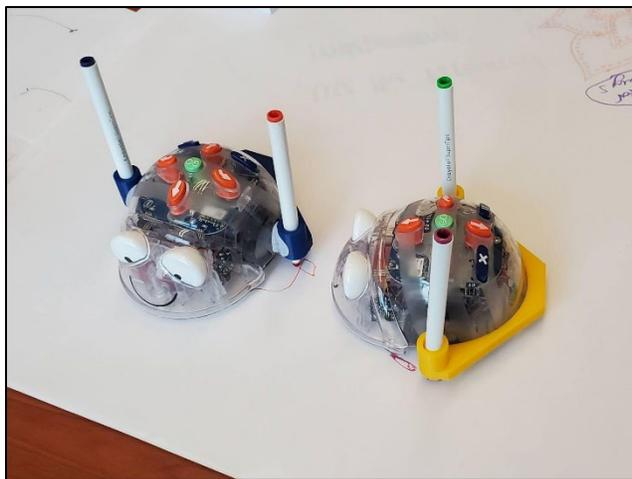
Figure 2. Bee-Bots with 3D printed attachment that holds two markers.
