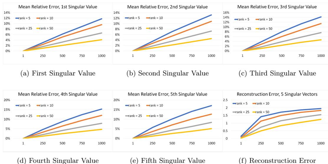
Figure 3: Mean relative error of the first five singular values and reconstruction error of corresponding singular vectors. X-axis is the number of observations processed.
