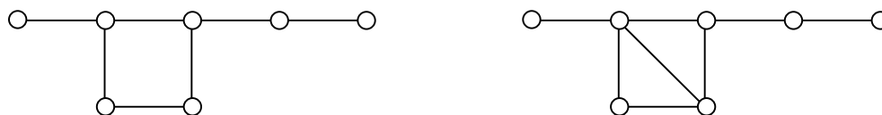
FIG. 4.1. An \mathbf{A} -controllable graph which is not \mathbf{Q} -controllable (left), and a \mathbf{Q} -controllable graph which is not \mathbf{A} -controllable (right).
